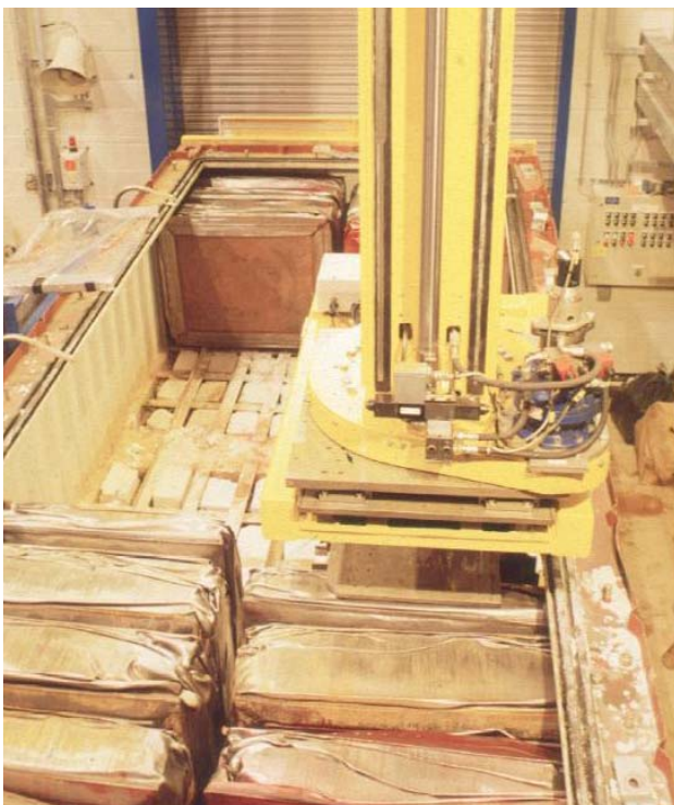
Compacted waste pucks being placed in LLW package.
