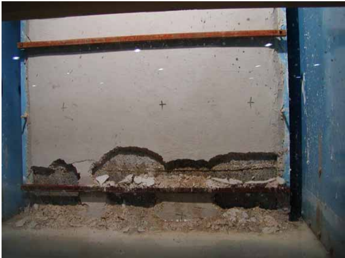
Photo 7.20 Wall MFF3 Collapse of lime plaster
