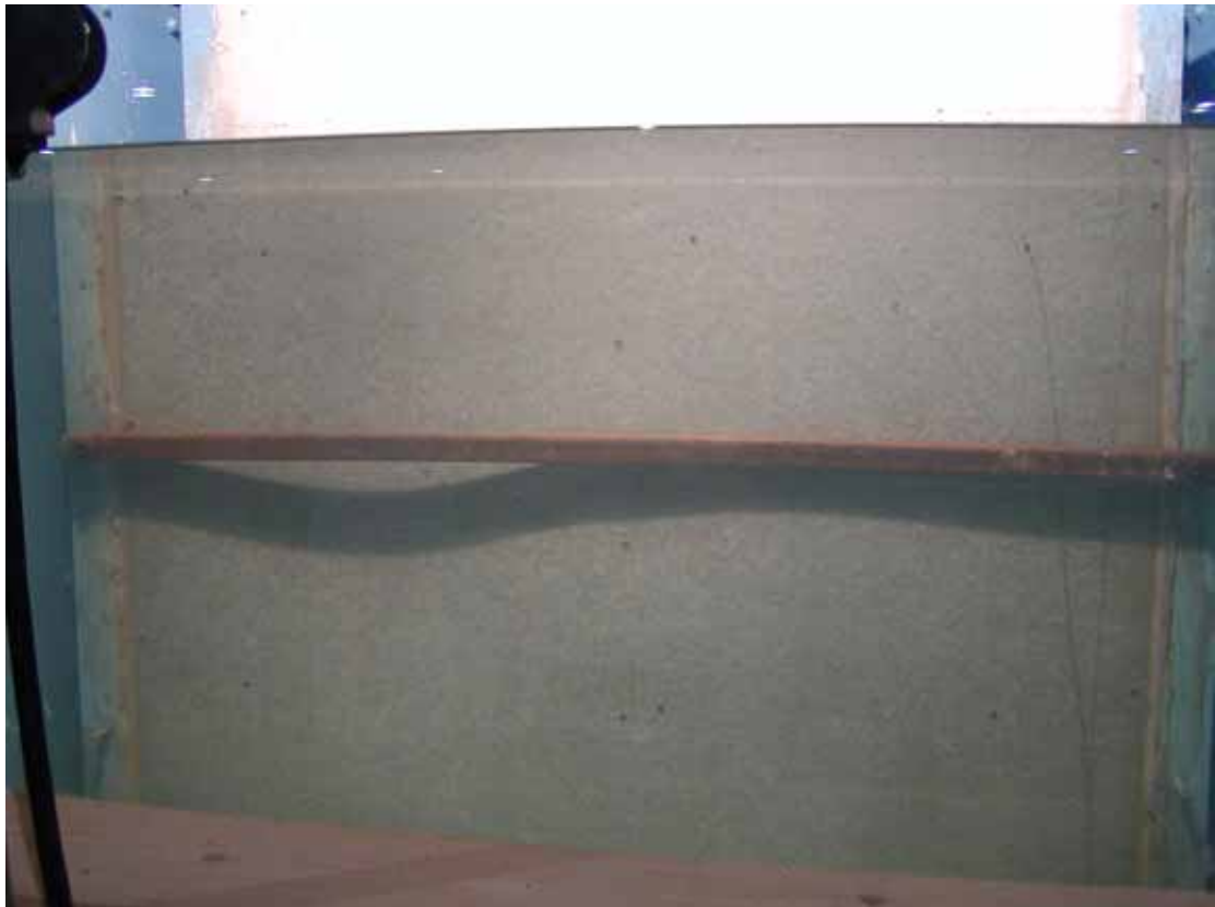
Photo 10.15 Wall S4.4 - Warped Fermacell board on internal face
