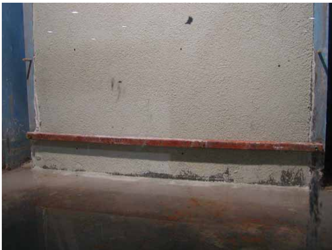
Photo 10.10 Wall S4.2 - Wall with external insulation; leakage
