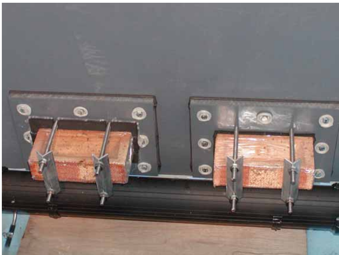
Photo 5.2 Wire cut bricks ready for testing
