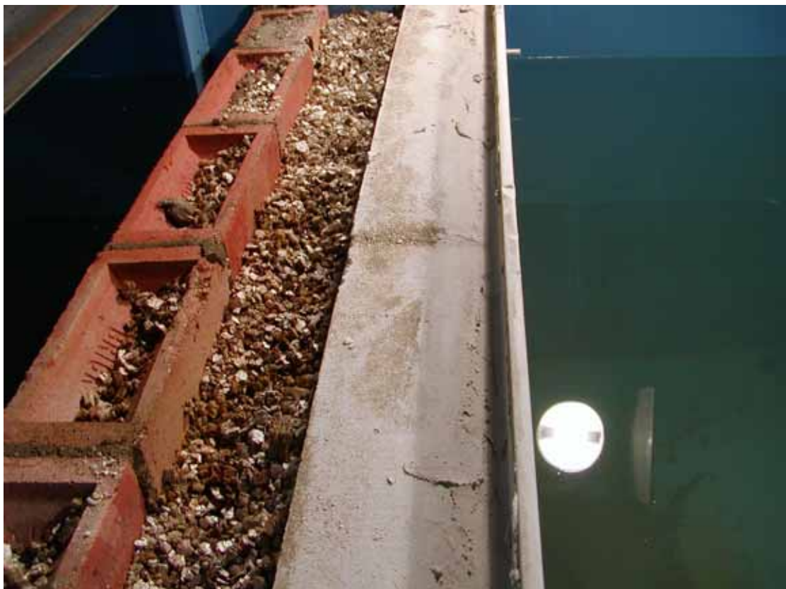
Photo 7.10 Wall MFF2 showing loose insulation in cavity after wet phase of testing
