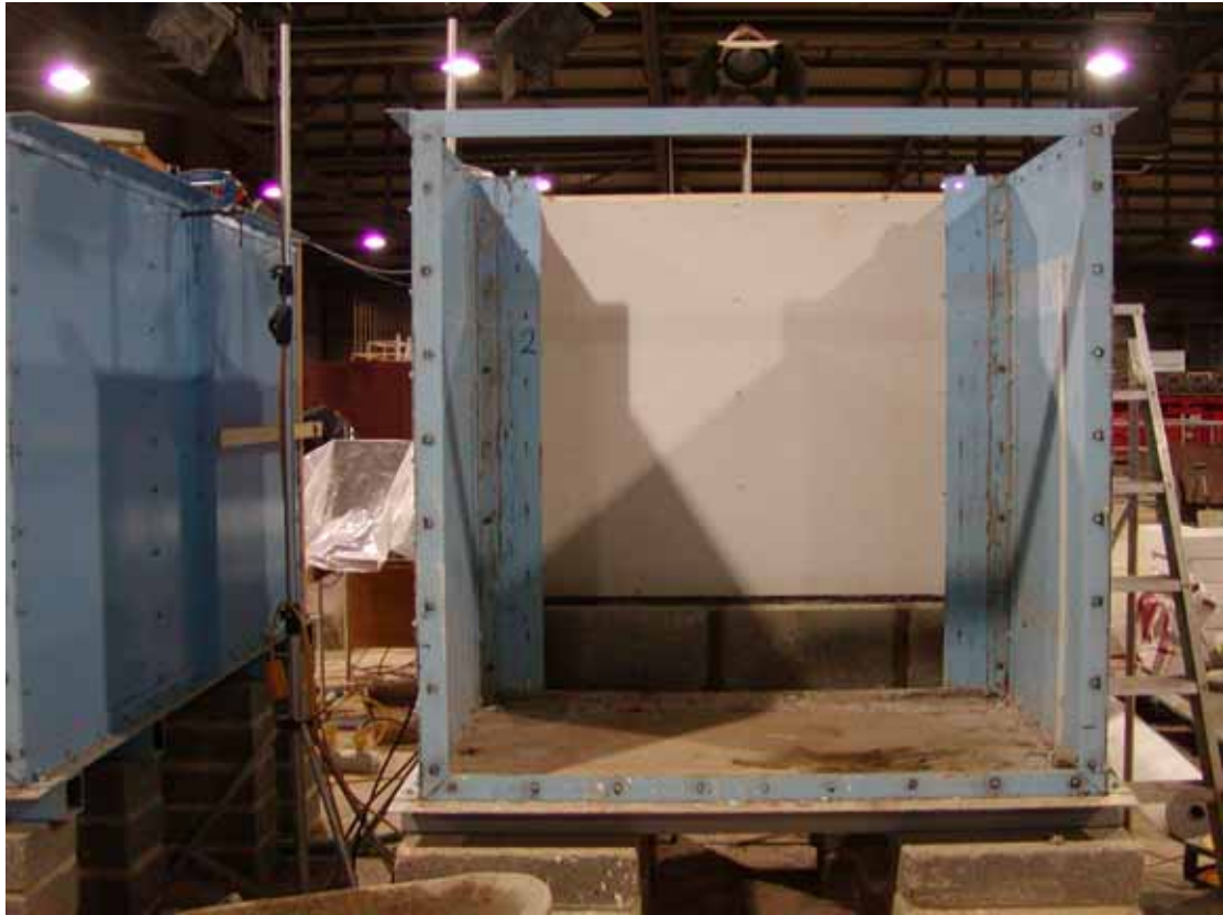
Photo 10.14 Wall S4.4 - Fermacell board replacing sheathing
