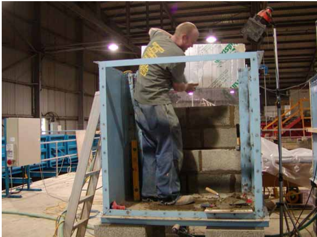
Photo 10.12 Wall S4.3 - Introducing insulation in the cavity
