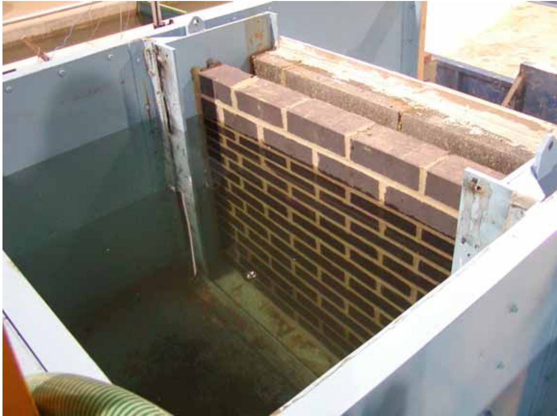
Photo 7.3 Wall ME1 during wet test
