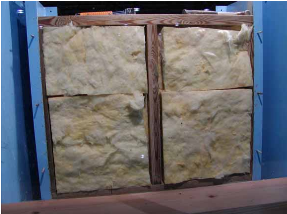
Photo 7.16 Wall TF1 being built showing insulation
