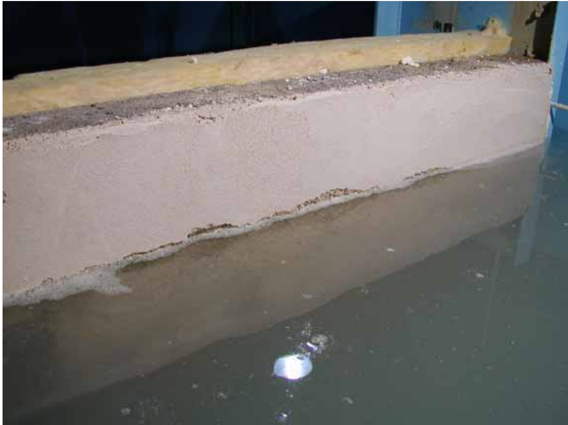
Photo 7.21 Wall MFF3 Cracking of lime plaster at surface water level
