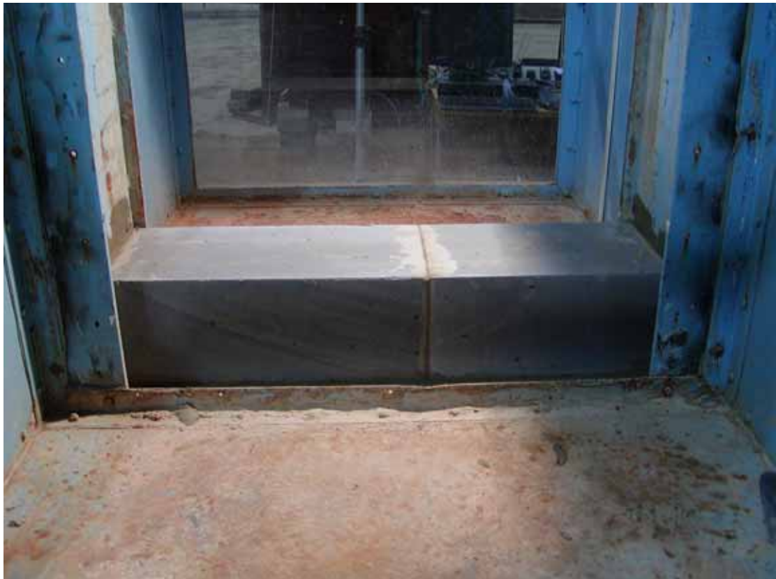
Photo 10.1 Wall S4.1 - Thin joint - first course
