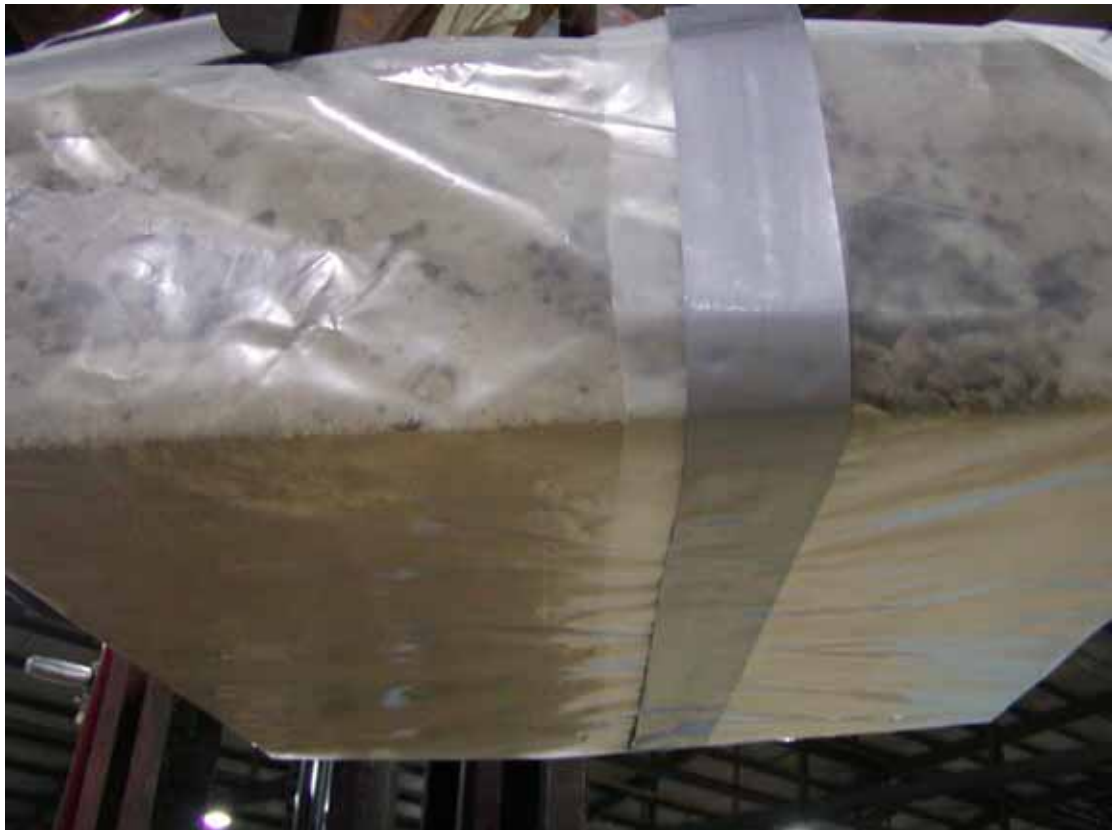
Photo 9.6 Floor Arrangement 5; taped membrane
