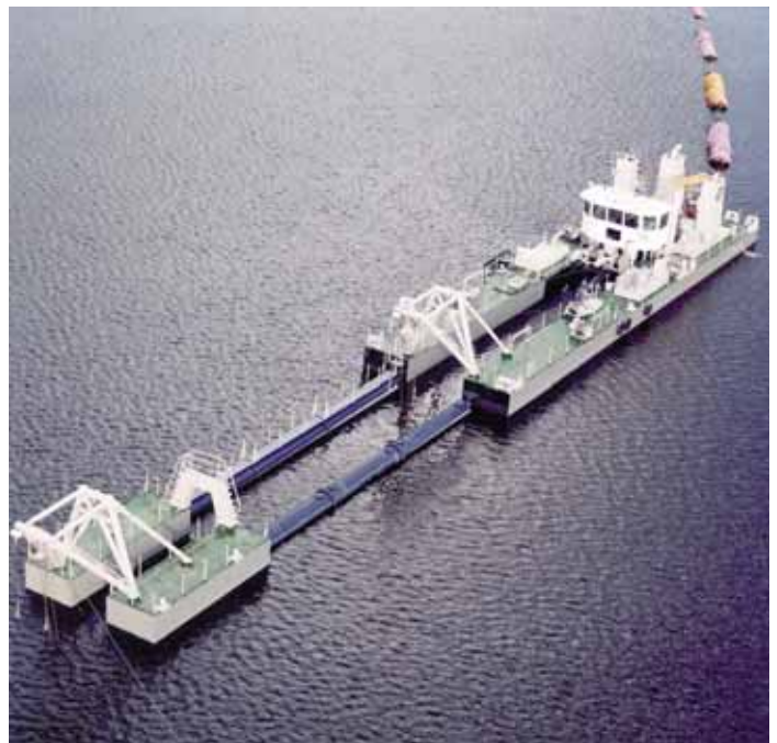
A suction dredger for winning sand at depth (courtesy Nick Bray)
